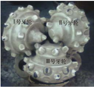
图 2 437 型牙轮钻头 Fig. 2 Tri-cone bit of Model 437
