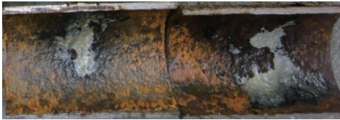
图 8 清水清洗效果 Fig.8 Cleaning effect with water
