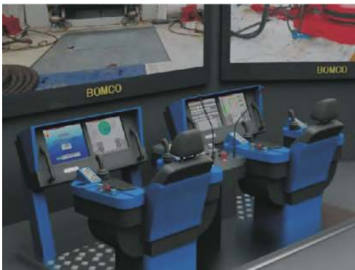
图 2 我国小型智能钻机的井口控制系统-双集成司钻系统 Fig. 2 Wellhead control system-dual integrated driller system for small scale intelligent drilling rig in China
